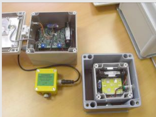
Fig. 26. Counter RBX5 L open. Transmitter, receiver and data storage device (yellow)
